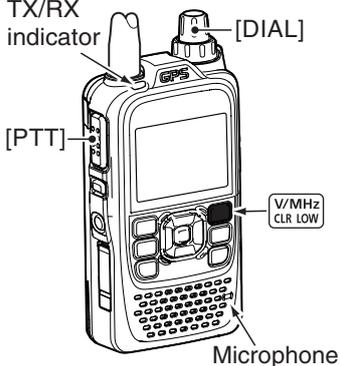
**WARNING! NEVER** transmit for long periods of time. During prolonged transmissions at high power or mid power, the transceiver radiates heat to protect itself from overheating. The transceiver’s chassis will become hot and may cause a burn.
